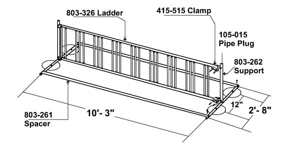
Main Frame, legs and spacers are 1 5/8'' O.D. hot galvanized welded pipe with 3/4'' O.D. hot galvanized ladder rungs. Spacing between tire posts is 3" center-to-center for small gap, 8  $\frac{1}{2}$ " center-to-center for large gap.
